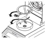
5 Place the sample pan handler with the inserted temperature adjustment disc with precision thermometer in the sample chamber.
