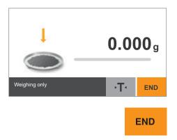
The weighing screen appears.You can now use the moisture analyzer as a simple lab balance.
