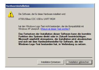
With 'Continue installation', the driver is installed. After that the Virtual Serial ComPort is available, in this example COM6. The COM number varies during installation.
