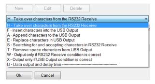
Various actions are available for data processing, some refer to **RS232 receive**, others to **USB Output**. You can recognize the reference by the fact that the corresponding text field is highlighted in green.
