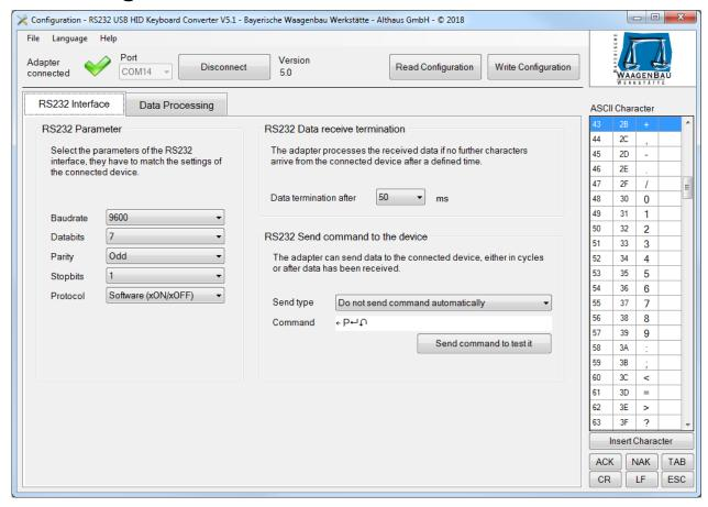
The configuration software for the RS232 USB HID Keyboard Converter can be found on the supplied USB stick in the directory "Konfigurationsprogramm und Dokumentation" as well as in the latest version on the Internet at www.bayernwaage.de .
