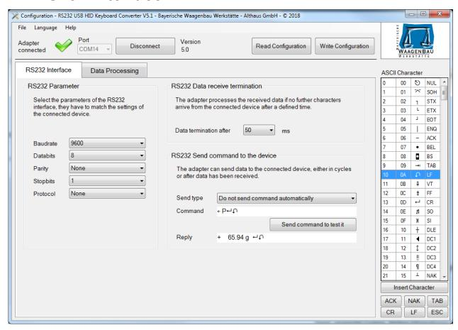
In the RS232 Interface configuration area you set the RS232 parameters of the connected device, specify when data reception is complete and have the option of sending a command to the device. Changes to these settings must be sent to the adapter via [Write Configuration] in order to activate them.
