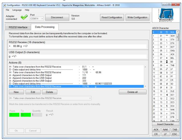
In the Data Processing configuration area, you can have the data received via RS232 from the connected device processed by the adapter before it is transferred to the computer via USB keyboard output. To do this, the adapter processes defined actions in sequence that lead to the desired USB keyboard output on the computer.
