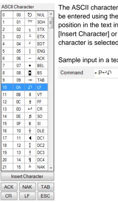
The ASCII character table is used to insert characters into text input fields which cannot be entered using the keyboard. To do this, place the cursor at the desired insertion position in the text input field, then select the character to be inserted in the table and click [Insert Character] or double-click on it. If you select a character in a text input field, this character is selected in the table.
