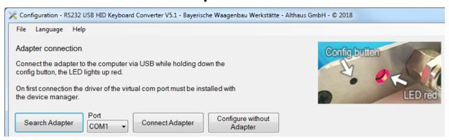
After starting the configuration software, you can choose whether you want to establish a connection or use the software without an adapter.
