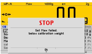
The maximum capacity of the scale can be increased retroactively. When the capacity is reduced, however, a message appears when the new maximum capacity falls below the calibration weight ("calibrated at").
