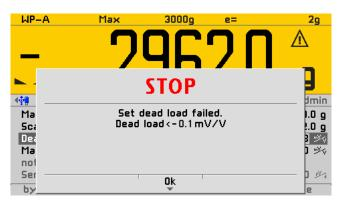
This message appears if the measurement signal is negative (load cells connected with wrong polarity or defective) when determining the dead load with [by load].
