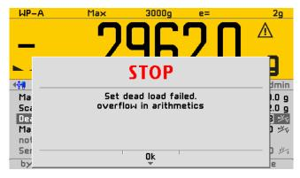
This message appears if the dead load entered in mV/V is higher than 5 mV/V.
