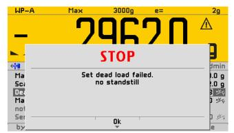
The dead load entered in mV/V plus maximum capacity in mV/V is higher than 3 mV/V (= 36 mV).
