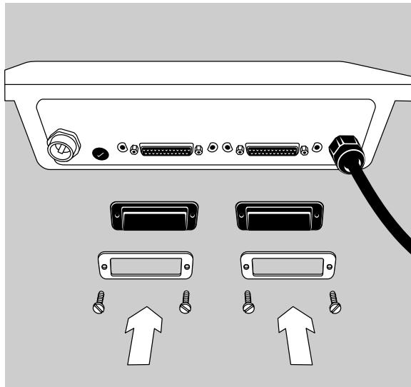
**Installation for operation up to a protection rating of IP65 with sealed interface ports**
