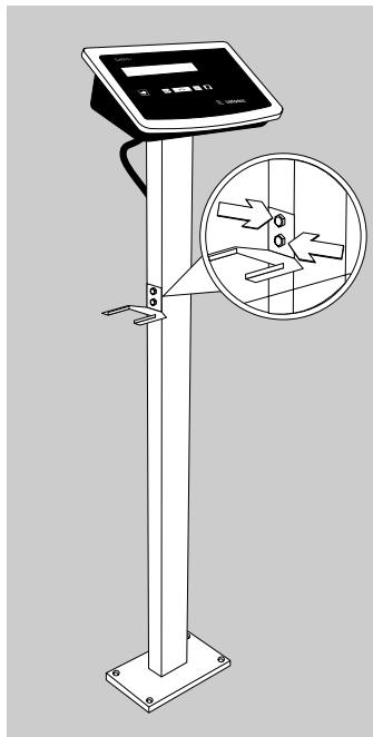
You can attach a retainer for a bar code scanner (YBH01CWS) to either side of the column.
