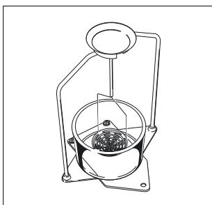
To determine the specific gravity of solids when their density is greater than that of the liquid in which the sample is immersed, use:
