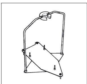
Always use the metal platform to hold a beaker. Please position this platform through the frame so it rests evenly on the base of the weighing chamber. If you are using a BA, BP, CPA, CP or ME balance, turn the platform so it rests on the pins which are far apart. For RC and MC balances, the platform should rest on the pins which are closer together.
