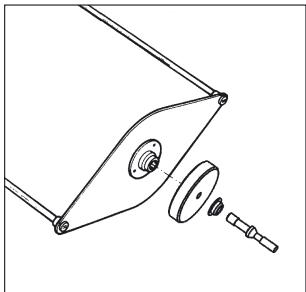
Screw the appropriate adapter into the underside of the bar frame base:
